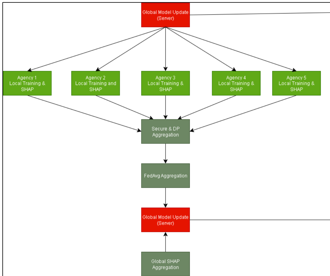
Fig.3: Threat detection system architecture
